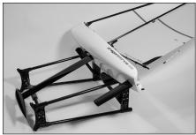
The Stand Upgrade Kit allows the boat to placed on the stand in the upright position for easy access when rigging and indoor storage (shown left), or the stand can be laid on its side and the boat secured in an almost horizontal position (shown right) for additional stability outdoors.
